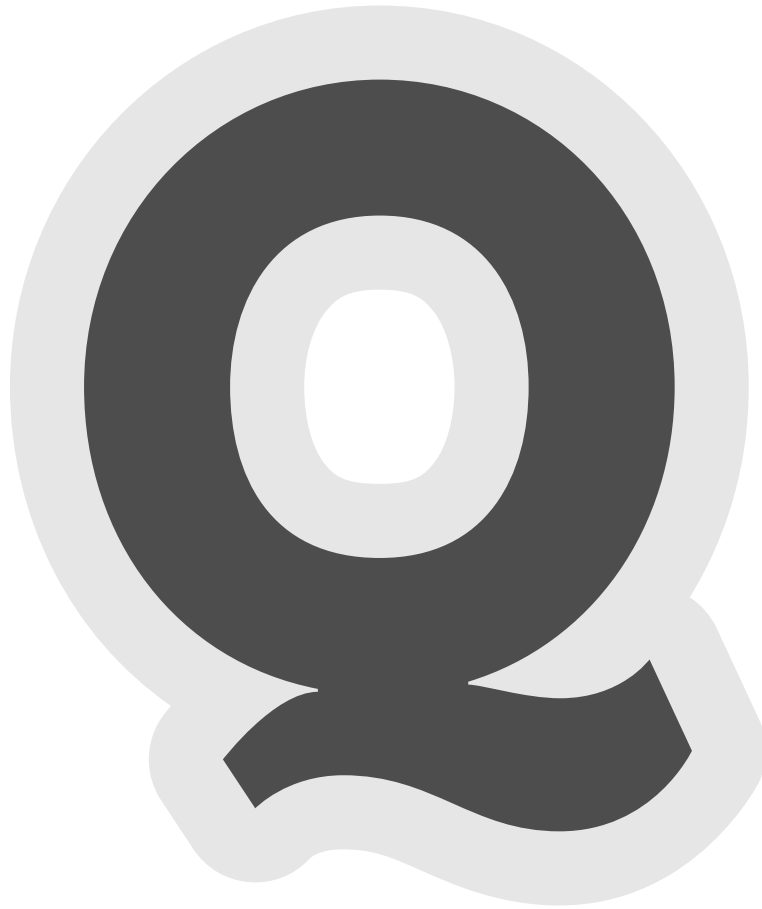
Figure 2: This path sequence forms the outline of the capital “Q” letter in the League Spartan typeface. The interior of the path sequence is represented in dark grey; as the two paths are oriented in opposite directions, the interior of the path sequence is included in \Omega . The interior of the inner path does not belong to the interior of the path sequence; a typographer would say that it is a closed counter of the letter.
