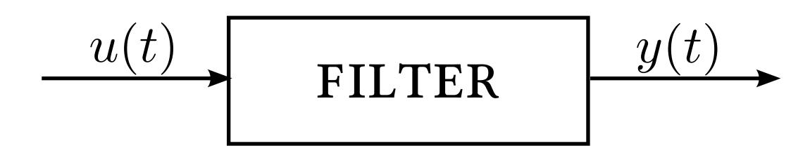
h(t) is the filter impulse response: y(t) = h(t) if  $u(t) = \begin{vmatrix} 1/\Delta t & \text{if } t = 0, \\ 0 & \text{otherwise.} \end{vmatrix}$
